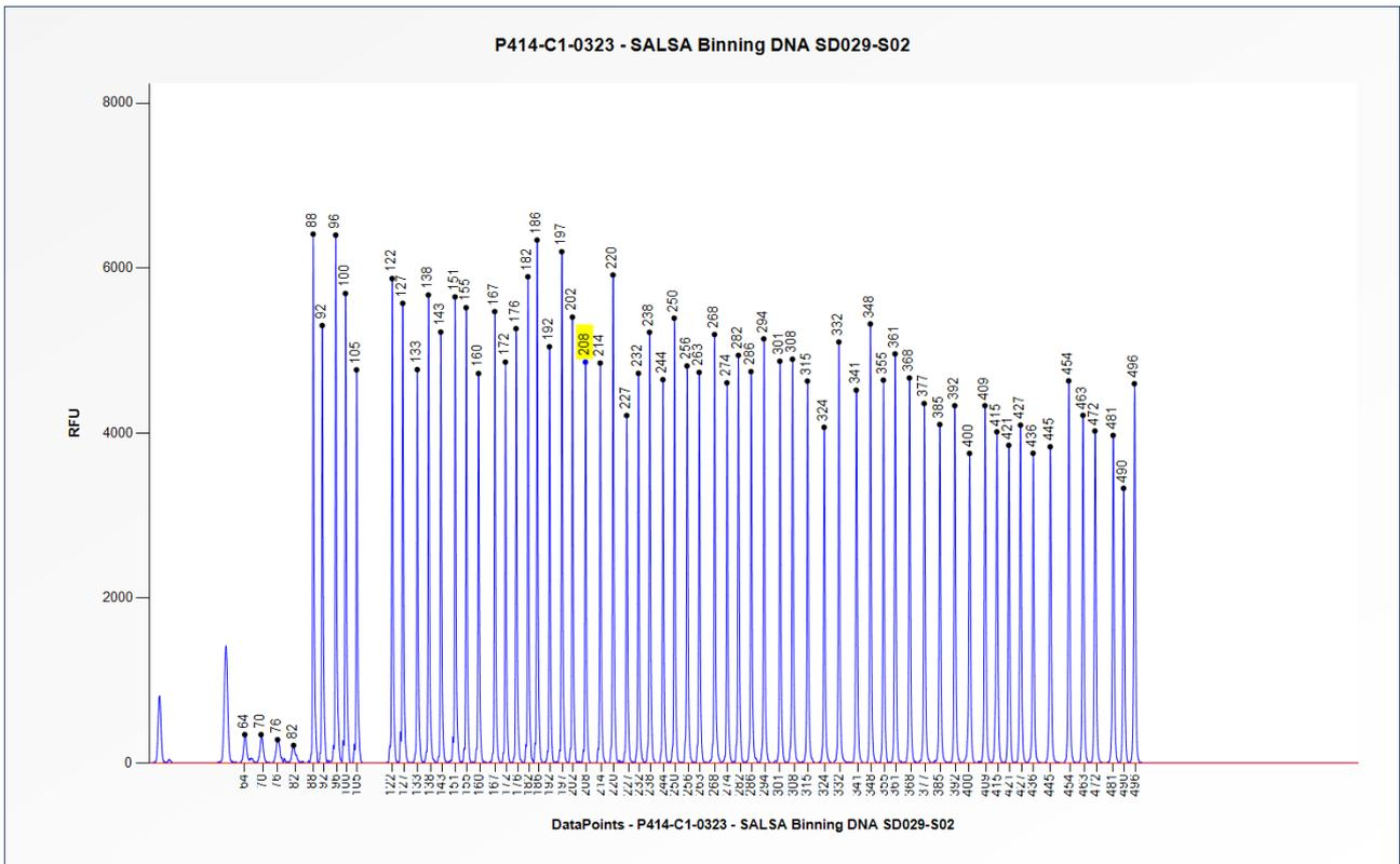
**Figure 3.** Capillary electrophoresis pattern from SALSA Binning DNA SD029-S02 (approximately 50 ng) analysed with SALSA MLPA Probemix P414 MDS (C1-0323). The location of the JAK2 p.V617F (c.1849G>T) mutation-specific probe at 208 nt is indicated.
