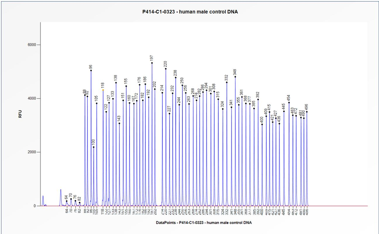
**Figure 1.** Capillary electrophoresis pattern from a sample of approximately 50 ng human male control DNA analysed with SALSA MLPA Probemix P414 MDS (C1-0323).
