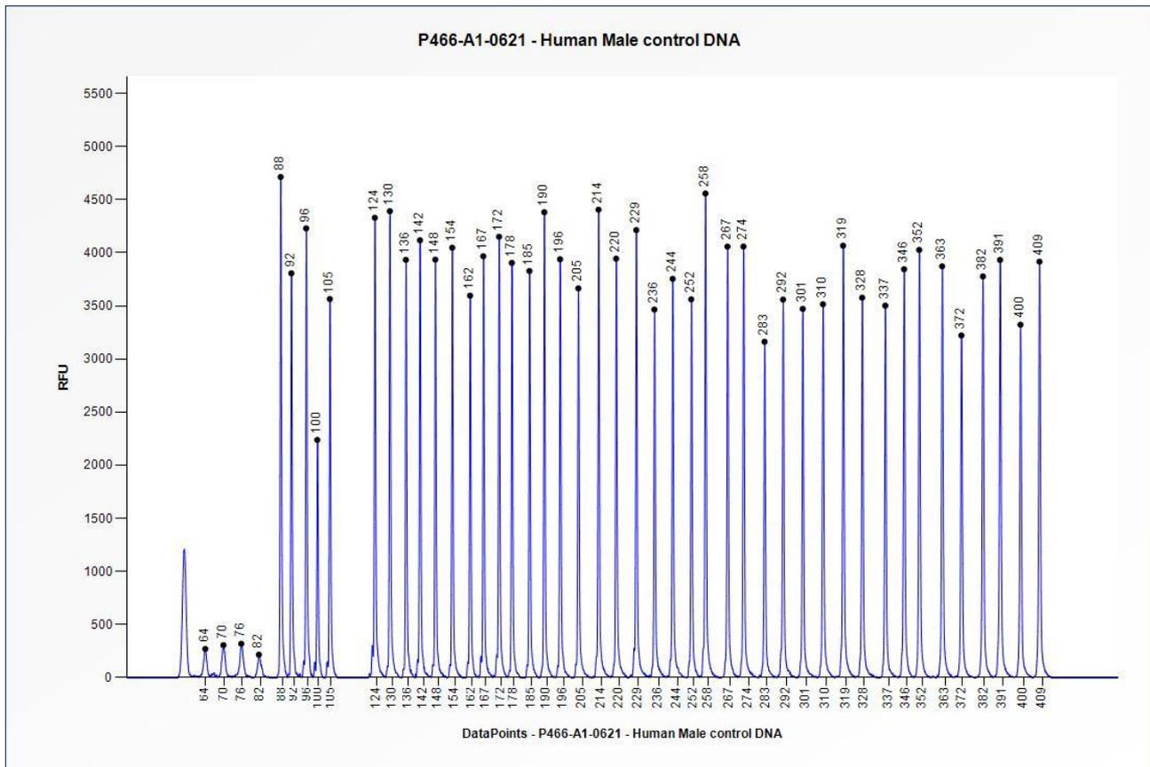
**Figure 1.** Capillary electrophoresis pattern from a sample of approximately 50 ng human male control DNA analysed with SALSA MLPA Probemix P466 CDC73 (A1-0621).
