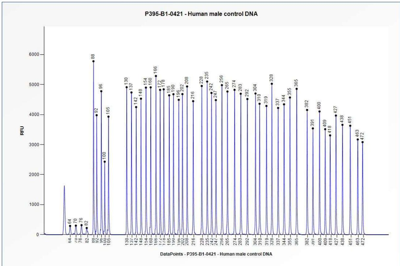
**Figure 1.** Capillary electrophoresis pattern from a sample of approximately 50 ng human male control DNA analysed with SALSA MLPA Probemix P395 MEF2C-FOXG1 (B1-0421).
